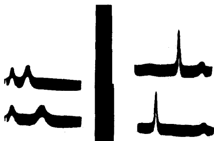
Fig. 1. Tiselius Electrophoresis of trout phosvitin b. Left: Ascending boundaries after 5' and 10'. Right: Descending boundaries after 11' and 24'. Perkin-Elmer Apparatus Model 38 A. 2 ml cell, 0.03 M sodium barbital-HCl buffer pH 8.6, 200 Volts, 10 mA, 9.6 \times 10^{-4} \text{ ohm}^{-1} \text{ cm}^{-1} .
